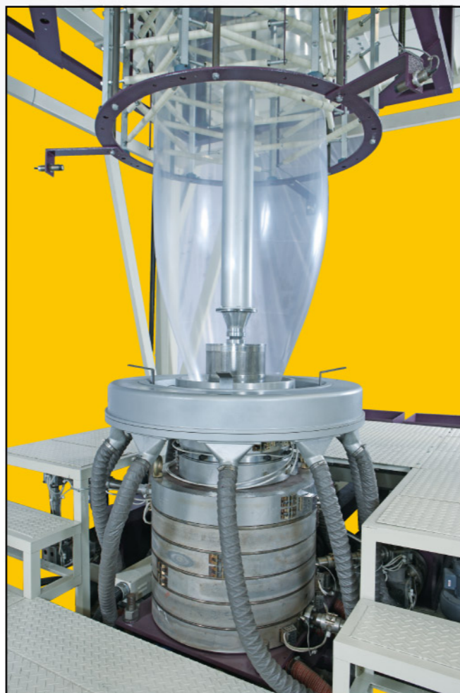
5 layer stack type die head + IBC Internal bubble cooling system + dual lip air ring
