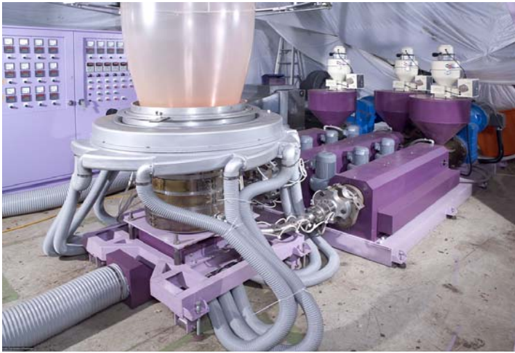
3 layer co-extruder with spiral type die head & dual lip air ring, auto loader
